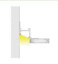
Corner recessed wall washer profile with opalised diffused cover.
